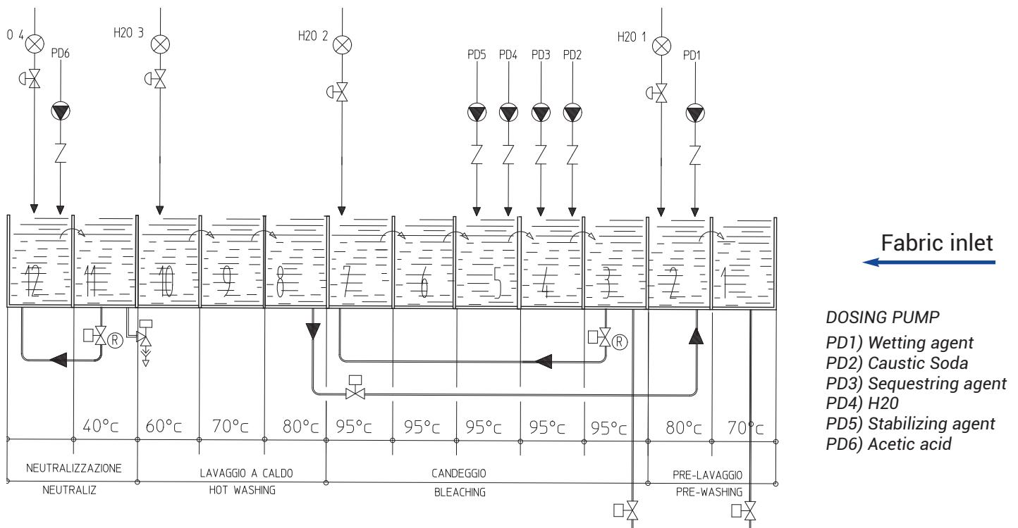
ALL WASHING LINES ARE AUTOMATED WITH TEMOELLETTRONICA SOFTWARE AND CONTROLLERS
