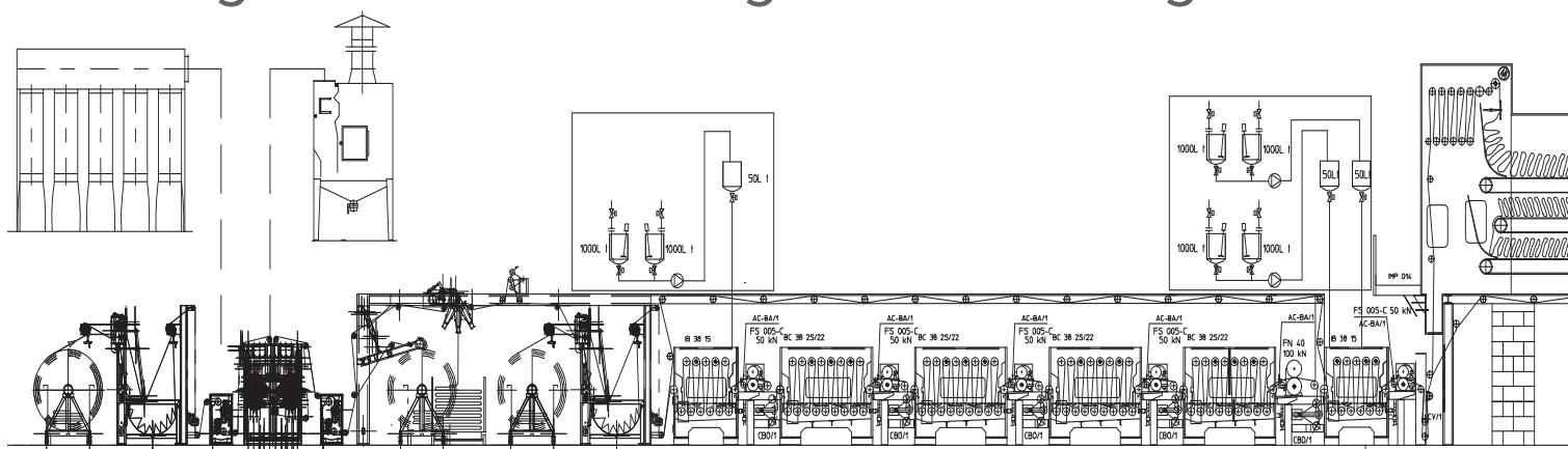
Desizing Unit + BC-38 Super + CS500 + Cylinders Dryers
